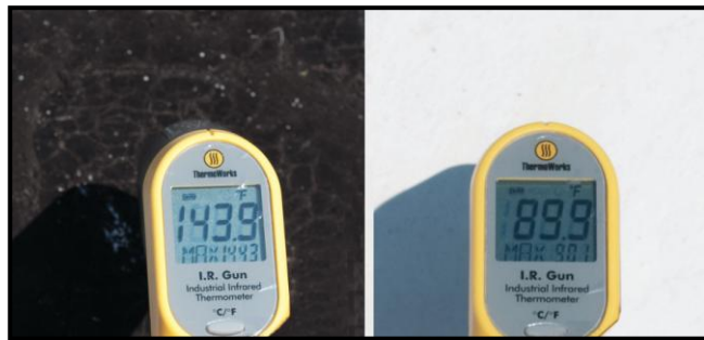
Figure 1: Dark vs. Cool Roof Surface Temperatures
